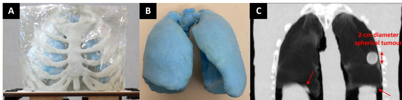
Figure 3: Images of the anthropomorphic thorax phantom designed at the University of Victoria. A: Photograph of the assembled thorax phantom. B: Photograph of a pair of foam lungs. C: CT images with breathing motion activated: motion artifacts are visible and indicated by red arrows and the spherical tumour has an oval shape.
