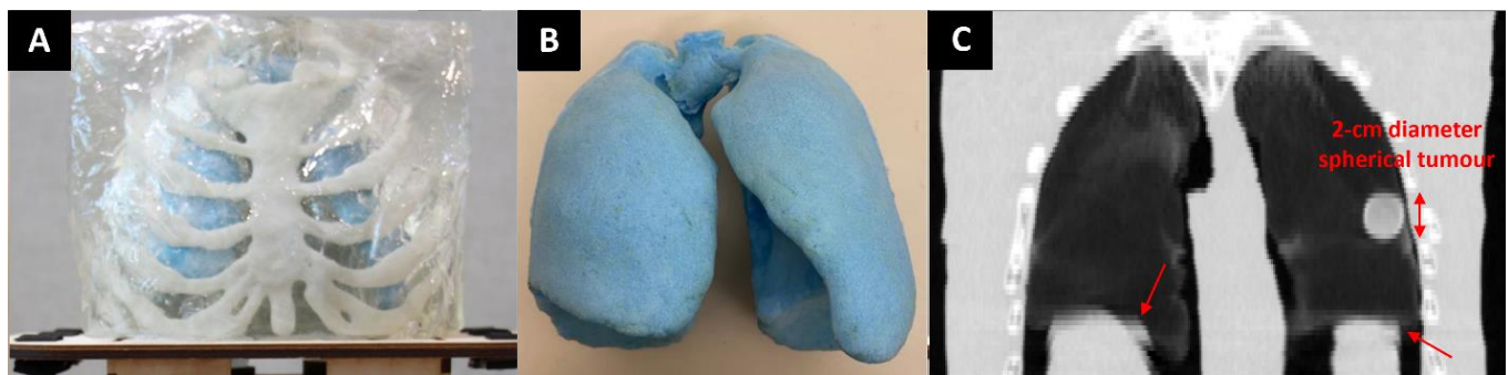
Figure 2: Images of the anthropomorphic thorax phantom designed at the University of Victoria. A: Photograph of the assembled thorax phantom. B: Photograph of a pair of foam lungs. C: CT images with breathing motion activated: motion artifacts are visible and indicated by red arrows and the spherical tumour has an oval shape.
